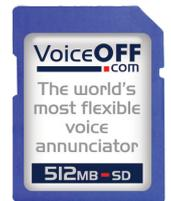
**Rename.** The audio files need to be in a folder called **SYSQ** and then renamed 0001.mp3, 0002.mp3 etc. so that the VoiceOff knows which sound to trigger with which alarm input. This is printed on the inside of the VoiceOff lid for quick reference.
